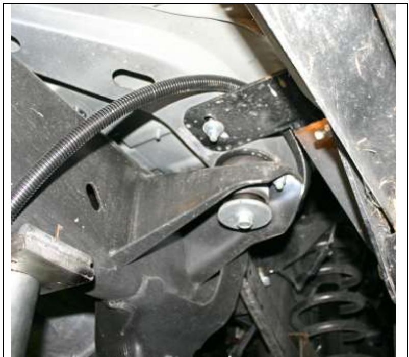
Route the snorkel wire through OEM stabilization brackets when possible.
